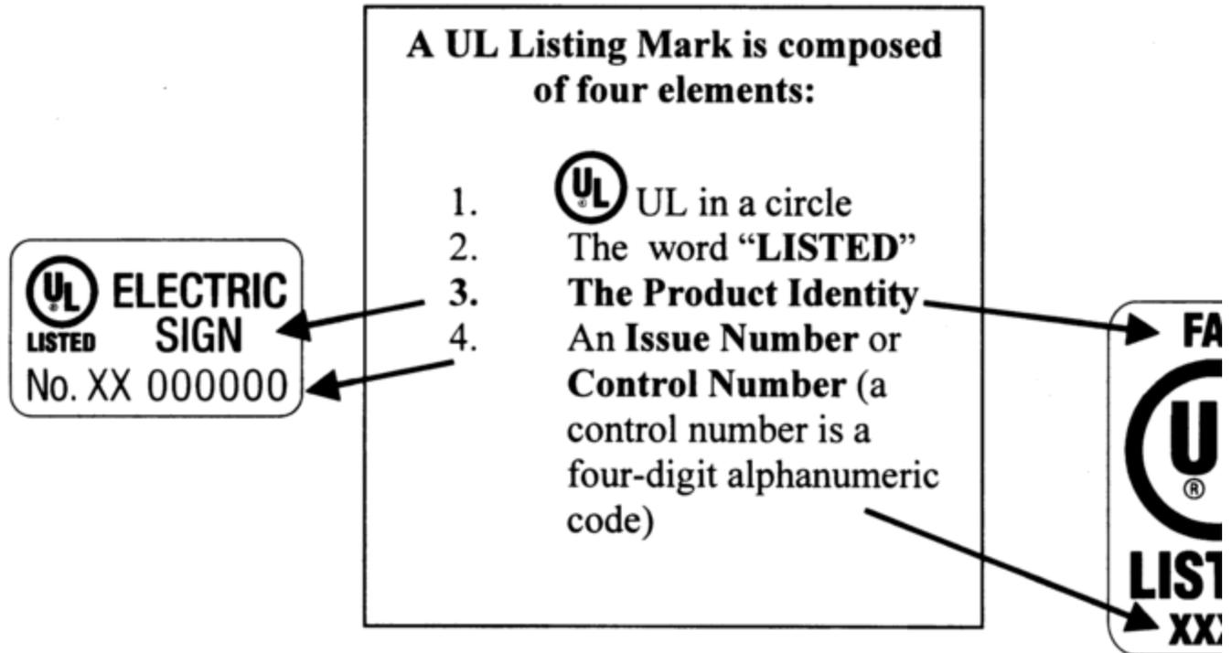
To answer your question on how the inspector would identify the equipment, item 3 is the product identity. To be considered a legitimate UL Listing Label, all 4 items are required to be on the label. As an example, UL Category QIKH (STATIC INVERTERS AND CONVERTERS FOR USE IN INDEPENDENT POWER SYSTEMS) on page 295 of the 2009 UL White Book under the topic UL Mark is very explicit as to what the product identity has to be.
